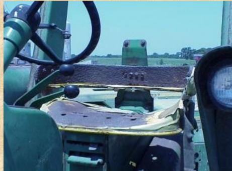
This cushion is worn to the metal. But the seat belt is still intact.
