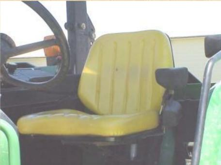
John Deere 6200 ergonomic seat: vacuum sealed vinyl cushion, armrests pivot vertically, backrest adjusts for support and positioning, fore and aft, seat belt retracts and adjustable weight gauge.
